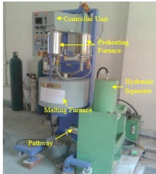
Fig: -Bottom pouring stir casting furnace with squeeze casting facility
